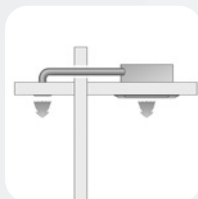
Air conditioning of an adjacent room
